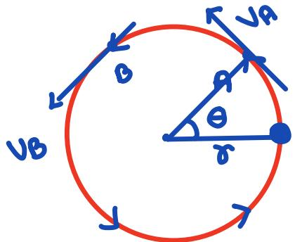
Angular velocity / =  $\omega = \left( \frac{d\theta}{dt} \right)$
